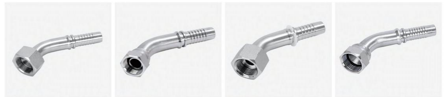
P/N:20741 45° metric female 74° cone seat P/N:22641 45° BSP female 60° cone P/N:24241 45° ORFS female flat seat P/N:26741 45° JIC female 74° cone seat sae
