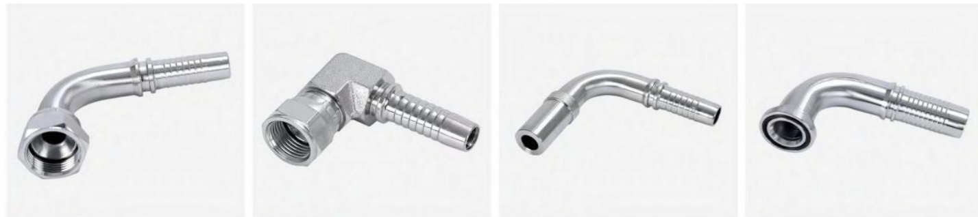
P/N:26791 90°JIC female 74° cone seat sae P/N:26791K 90°JIC compact female 74° cone seat sae P/N:50091 90°metric standpipe straight P/N:87391/87691 90°Sae flange 3000psi/6000psi
